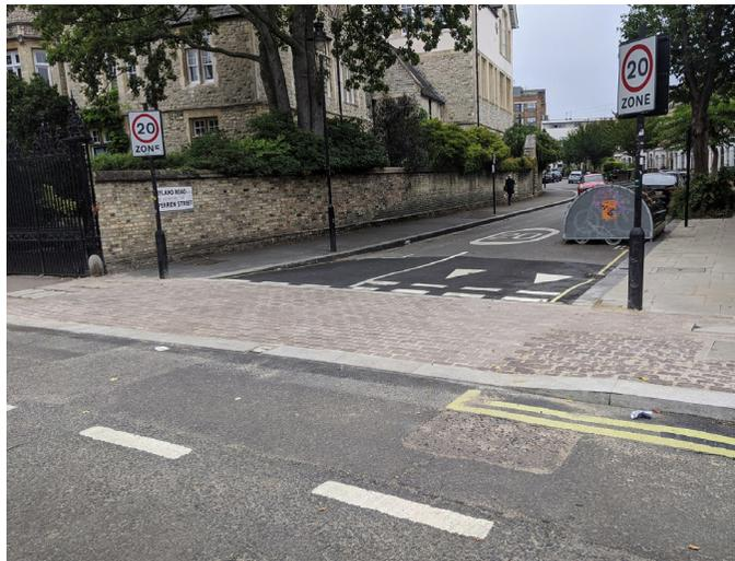
Figure 86: Continuous paving material and height across the junction.
