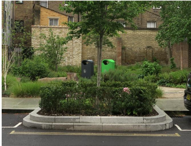
Figure 88: Kerb build out with street greening and a double kerb to prevent vehicle overrun.
